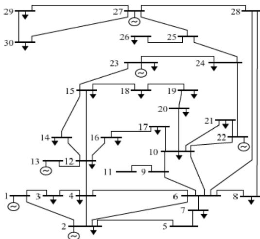
Fig.3: Single line Diagram for IEEE 30-bus Distribution Network
